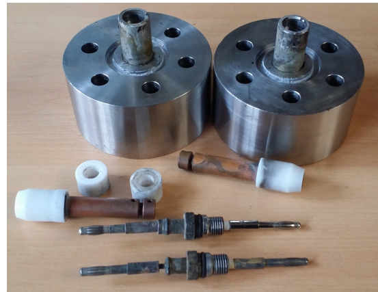
(b) Constantan wire holders pieces, note the wear in the plastic (white) piece.
