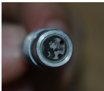
Figure 1.5: Pressure sensor for the test Bombe cover in Constantan dust.
