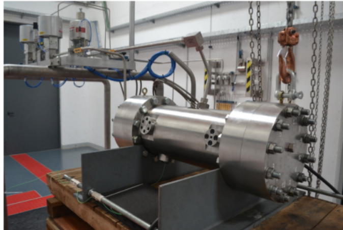
Figure 1.2: Outline design (top) and view of the Bombe and its associated gas filling system (bottom), in [1].
