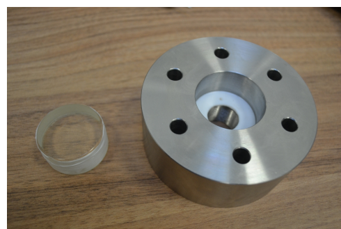
Figure 1.6: Laser window for the test Bombe, fused-silica round-window (left), support and chamber lid (right).
