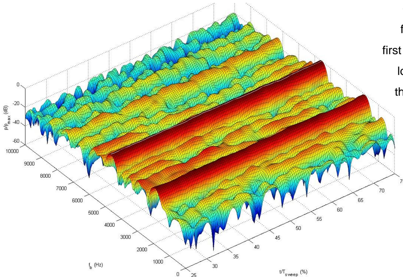
← Spectrogram obtained from a calibration test for first prototype, using a much lower frequency rate than that being tested currently and on monostatic antenna configuration
