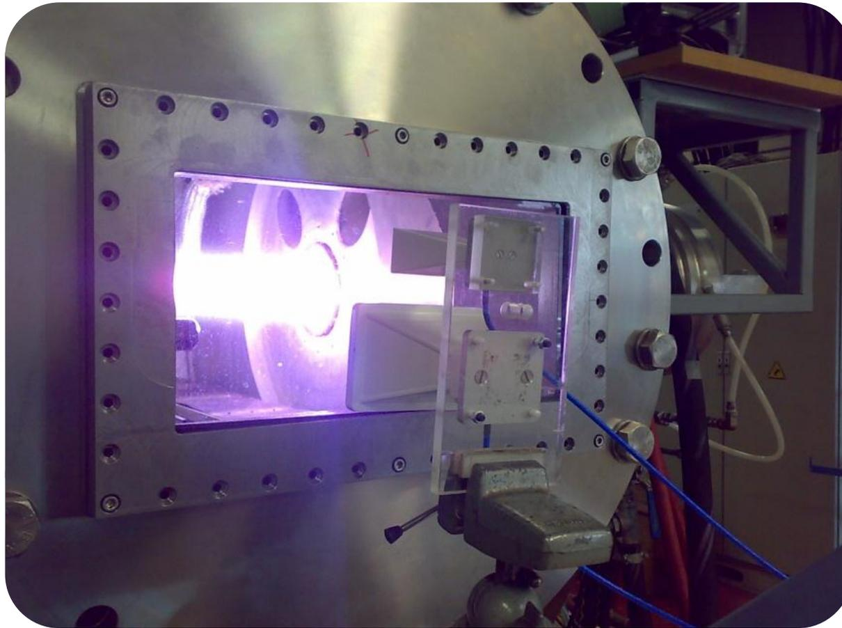
← Preliminary test conducted on the Plasmatron facility at VKI, to determine if it could be observed reflections from the plasma for the probing frequency range of 12 GHz to 18 GHz
